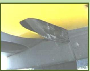
a higher speed than usual. The scraping noise was horrifying!! However the aluminum strip I added took the punishment not the skid pad. Fortunately there were no cracks or bent tubing!
