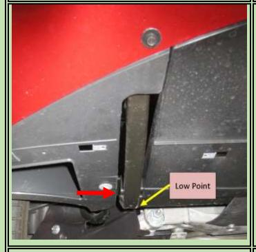
This is a picture of the "skid pad" in the C7. Unlike the C6, there is a gap on either side so it was easy to remove the paint and "roughen" the surface as suggested in the instructions. It was easy to gain enough access with the oscillating tool to quickly do most of the job.
