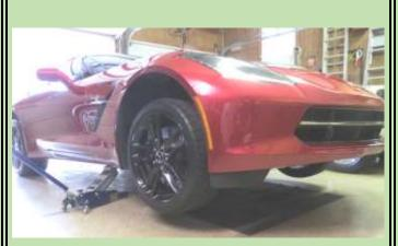
The car does not have to be jacked up very high as the skid pads are close to the front. It is advised to put jack stands under the car whenever it is jacked up. In this case they can be placed under the front cradle as defined in the Owner's Manual. Since you will not be going under the car very far just placing the jack stands under the outer ends of the cradle it all that is necessary.
