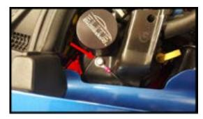
**Step 6:** Use a # 15 torx to remove the 3 screws behind the splash shield. Pull back the inner fender panel to get to the cove area. Place a light inside the fender to guide the led strips in place.
