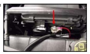
**Step 4:** On Z51 or Z06 cars you can use the 10mm bolt on top of the oil tank for the ground wire. Non Z51 cars, route the black wire along the plastic piping going towards the alternator (white arrow). Secure black wire on the ground terminal below the alternator (red arrow) using the supplied nut. This is where a magnet comes in handy. Its easy to drop the nut.
