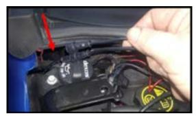
**Step 10:** Wipe the mounting area a couple inches away from the vent for best results. Apply the adhesion promotor then peel the backing off the strip and mount it as shown. It's not easy so be patient.
