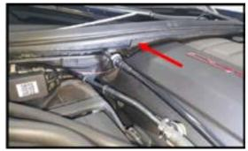
**Step 13:** Now you can mount the hood vent strip. Wipe the mounting area with the supplied alcohol pads. Apply the adhesion promotor to the edge of the ducting. Position the strip as shown. Center the strip on the ducting so the wire comes out as shown in the next picture. Be sure to work the strip into the center and corners as this is the most likely place for it to want to pull off. Keep working it until it fits the corners well.
