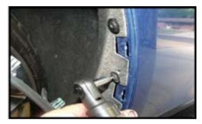
**Step 8:** On the passenger side guide the led strip and the extra lead down into the cove area. Use the light as a guide. This shows a Z51 car where it goes behind the oil tank near the coolant tank.
