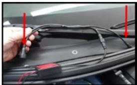
**Step 14:** To secure the wire in place drill a 1/8" hole in the ducting below the wire and use a wire tie to secure the wire to the ducting. You can use more than 1 tie if you wish.
