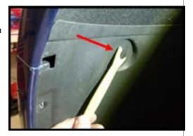
**Step 5.** Pull back the small white locking tab to remove the side marker connector.
