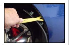
Step 2. Remove the 3 torx #15 screws so you can tie back the inner fender panel as shown to gain access to the cove.
