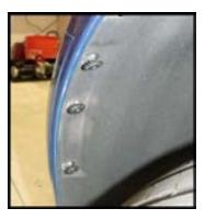
**Step 4.** Also remove the retainer shown here. Pry out the center of the retainer so you can remove it completely. Tie back the inner fender panel to gain access to the side marker light housing connector.
