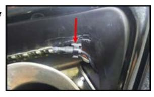
**Step 16:** This is looking down through the tailight opening to show where to mount the side led strips. Mount them a couple inches forward of the vents. Wipe with alcohol then apply adhesion promotor sparingly. Center the strips in the openings and peel the backing off to apply. Always tape the cables to the panel to prevent the strips from pulling off (red arrows). Repeat on both sides.
