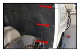
**Step 2:** The inner fender panel is very flexible so you can untuck it from behind the fender then lift the bottom up and out to gain access to the rocker panel area to fish the extension cable from front to rear.
