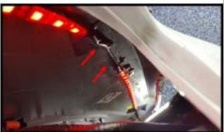
**Step 17:** Now go back and tape down the cables wherever you can. We tape them to the bottom of the rear fascia where the cables go out to the side vents. Wipe the panels first as they will be dirty. Finally bundle the extra cable and tie it up away from the exhaust system.
