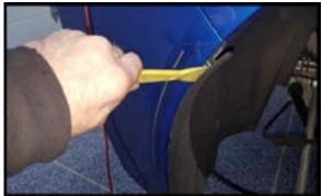
**Step 12:** Looking through the quarter panel you can see the lower rear grills. There are 3 tabs on each side you need to release to remove it. Release the bottom ones then pull out while you release the rest of them. Get the top 2 through the tailight opening.
