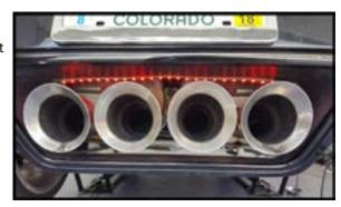
**Step 15:** Remove the backing from the cable clips before you stick the ends of the led strips. Be sure to prep this area with adhesion promotor. Come back and press the clips in place after a few minutes.
