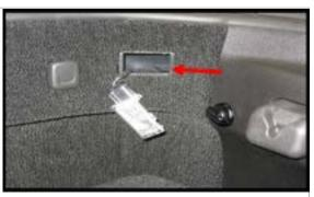
Step 2. Pull up on the weather strip so you can route LED wires behind the panel and through the light opening (red arrow).
