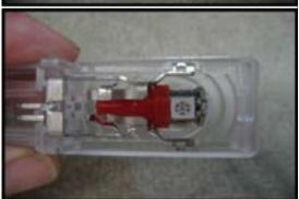
**Step 4.** If you are still having trouble getting it to light make sure the factory contact (red arrow) is contacting the small led wire (blue arrow). If they are not contacting each other you can move one or both of them to get contact. After all is working re-install the housings and enjoy the new lights!
