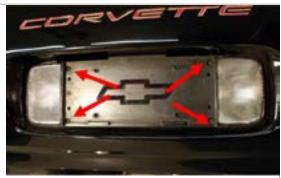
Step 2. Cover the area below the housing before you lay it down to protect your paint. Press the locking tang in and turn the socket 1/4 turn counter clockwise. Remove the bulbs by pressing them in and turn 1/8 turn counter clockwise.
