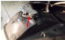
**Step 3.** Line up the pins on the LED housing with the channels in the socket. Push it down and turn it 1/8 turn. If it won't turn 1/8 turn, pull it out and turn it 180 degrees. Now push it in and turn to lock. Now test them by having someone put the car in reverse and hold the brake. If any don't light make sure you have them locked in properly.
