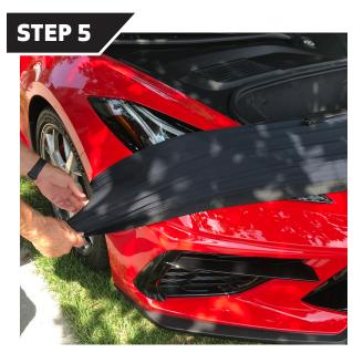
Stretch the mask across the front of the bumper, being careful not to rub the plastic clips against the paint. Attach the 4 snaps to other side of the car and the remaining 2 snaps on the original side.
