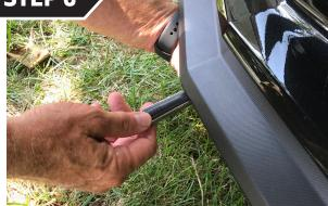
Pull the bottom edge of the mask down under the bumper, noting the position of the snap on the bottom-center edge of the mask. Replace the screw on the bottom of the bumper that best aligns with the snap on the mask with a snap head screw stud. Fasten the snap on bottom of the mask to the screw just installed on the bottom of the bumper.
