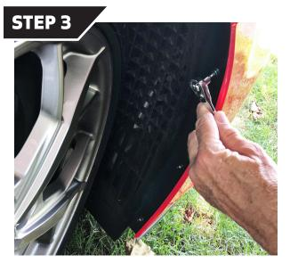
Locate the four (4) mounting screws at the edge of the bumper inside the fender liner and remove them. Replace each one as you go with the supplied snap-head screw studs. Repeat this step on the other side of the car.
