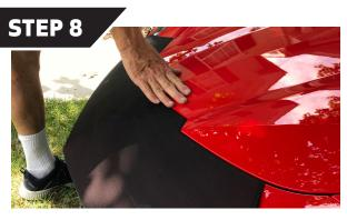
▲ **Note:** When closing the frunk, make sure the top edge of the mask does not cover the latch opening or in any way interfere with the full and secure closing of the frunk.
