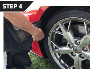
Begin the mask installation by fastening the top 2 snaps on one end of the mask to the screws just installed on the edge of the bumper.
