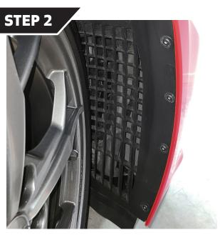
Turn the front wheels to gain easier access to the fender liner mounting screws that you will be replacing.
