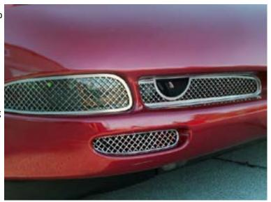
appropriate grille into the hole setting it against the black trim as you slide the top of the grille past the painted surface directly onto the black fog light shroud. Press firmly to set both the top and the bottom of the grille.
