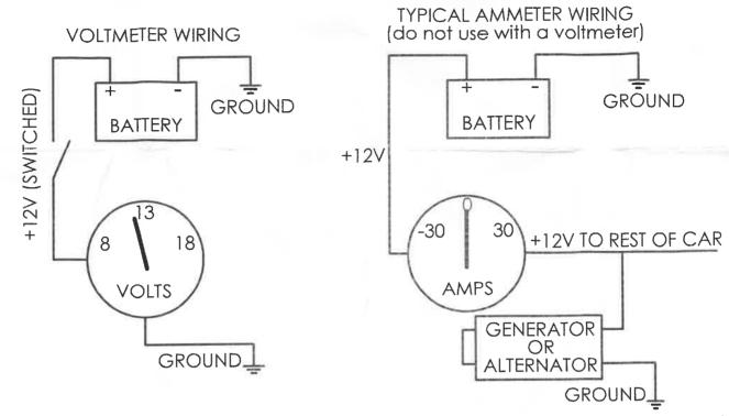
A voltmeter and ammeter are connected differently. If stock wiring is used, all of the electric current used by the car will pass through the voltmeter and cause permanent damage to gauge internals.
