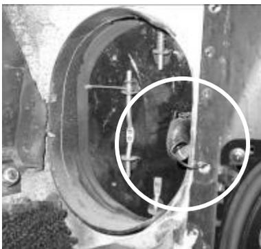
Using the existing spring. Attach the end over the hole as shown. This will keep the fresh air door closed.
