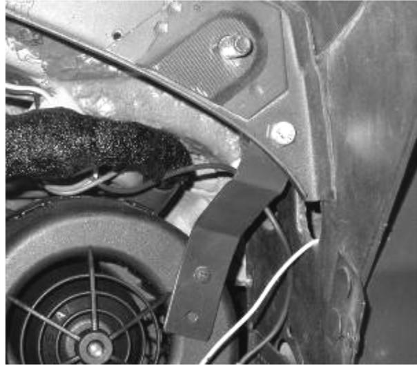
The picture below shows the power pack installed in the vehicle.
