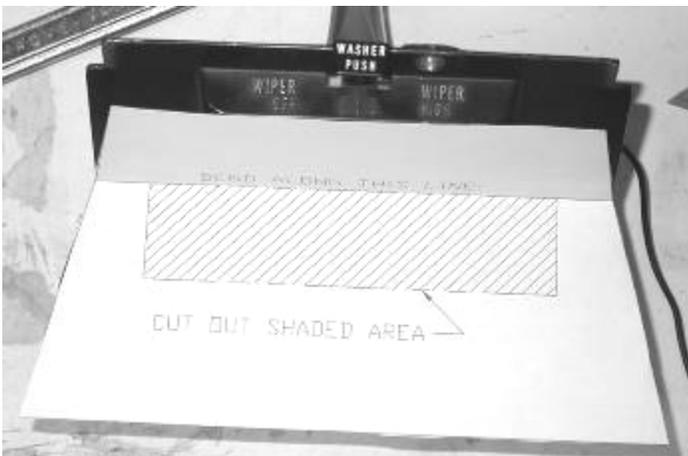
**CAUTION: CUT CAREFULLY. CHECK THE LOUVER ASSEMBLY FOR FIT. IT MAY BE NECESSARY TO FILE THE OPENING TO SIZE.**
