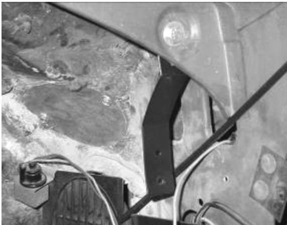
Locate blower support brace, (1) 1/4"-20 x 5/8" hex head screw, (1) 1/4" flat washer and (1) 1/4"-20 flange nut from the hardware sack kit.
