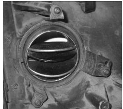
Attach the hose adaptor over the ball louver and retain with the (2) hold down brackets and the original hardware.
