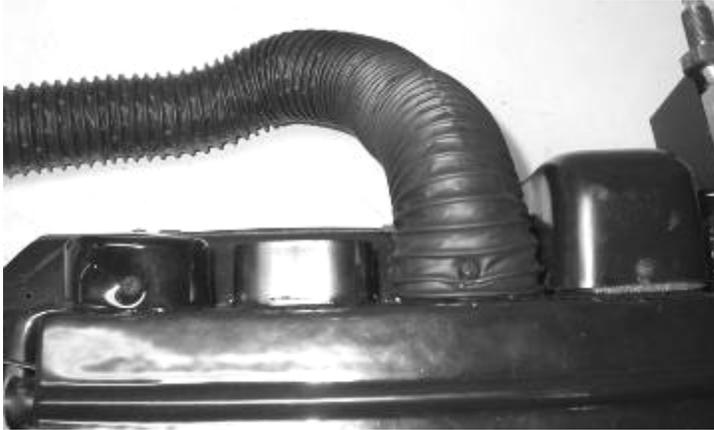
Locate the 2" dia flex duct and cut 21" from the 8 ft duct.
