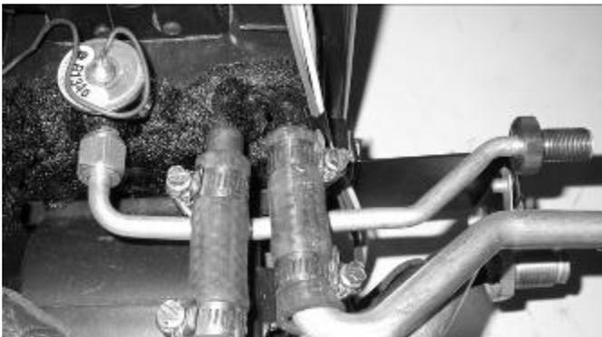
Locate in the hardware sack kit the #6 liquid tube and (1) #6 o-ring. Attach the tube to the expansion valve using (1) #6 o-ring and a few drops of mineral oil. Tighten securely.
