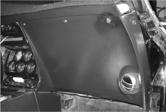
Attach the end of the 16" duct hose to the 90 deg hose adaptor on the dash cover. Reinstall the dash cover using the original hardware.
