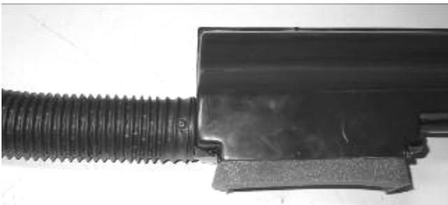
Locate the centre air distribution assembly and the 2" dia flex duct and cut (1) piece 36" long. Attach to the left outlet using (1) #8 x 3/8" pan head screw.
