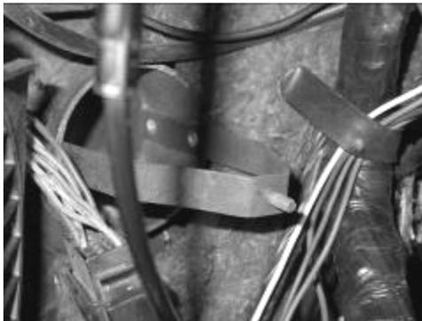
Locate the fresh air cover and slide over the inlet flange. Attach using the original wing nut.
