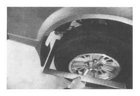
**STEP 3.**Remove tire if necessary and fasten the guard where any existing wheel well holes line up with the flare holes using metal screws and clip nuts.
