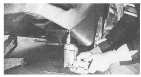
**STEP 4.**Drill remaining wheel well and bottom fender holes using a 9/64" bit. Install remaining self tapping metal sheet screws.
